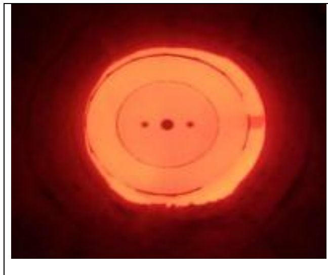
Figure 11.7: Typical picture of combustion obtained with a flameless burner
