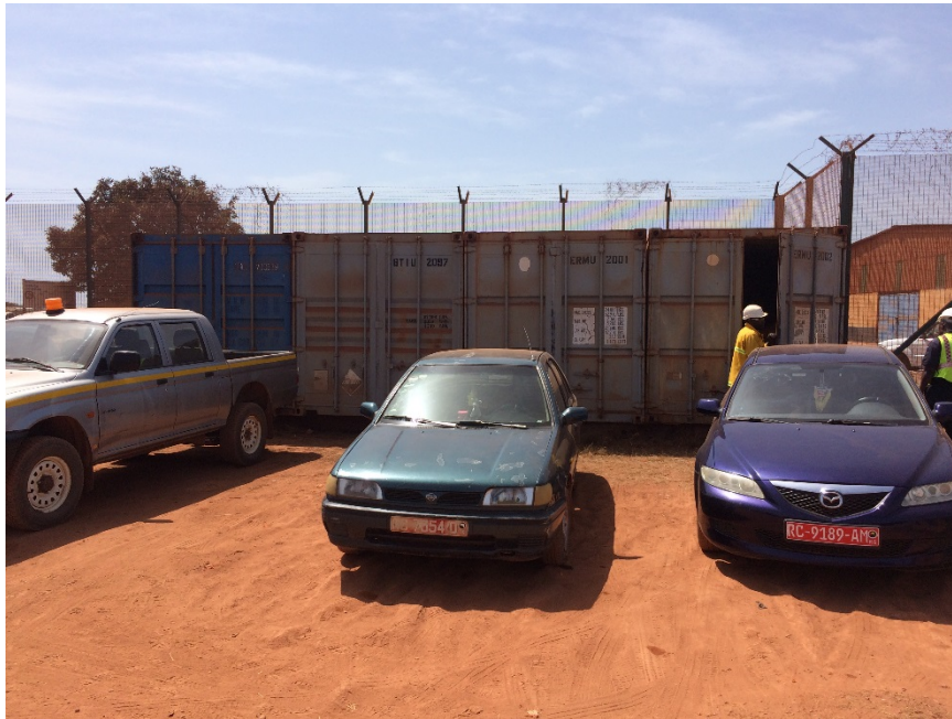
Photo 21. Container with oil spill response equipment – access blocked by parked cars
