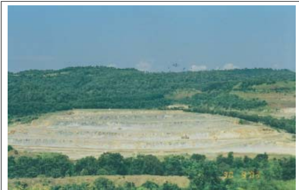
Systematic bench formation in a Limestone mine. Rehabilitated waste dumps are seen in the background— Chandrapur District, Maharashtra State
