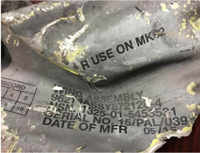
Remnant of a Paveway IV Guided bomb that struck the Hodeida Warehouses. The stock number indicates that Raytheon manufactured the bomb in 2015, after the start of the war. © Priyanka Motaparthy. Human Rights Watch
