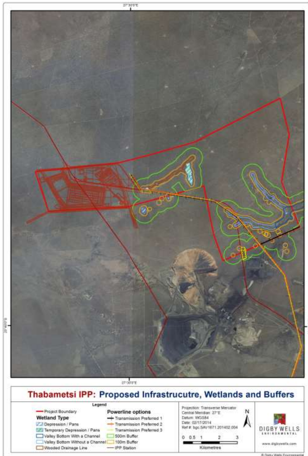
Figure 7.3: Delineated wetland areas within the project area, the proposed infrastructure and the appropriate wetland buffer zones
