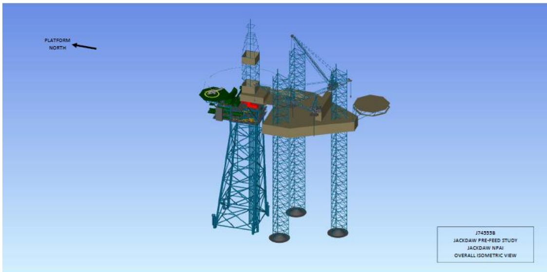
Figure 2-7 Example WHP view with Jack-up on station.
