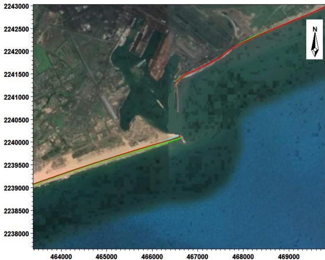
Figure 2-9 Shoreline change at Zone-1. Baseline conditions after 1-year (blue colour), Layout condition after 1-year (red colour) and Layout condition after 5-years (green colour)
