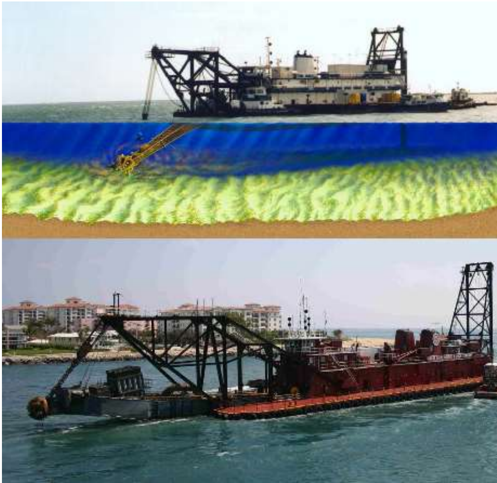
Figure 4: Cutter –suction dredger – Dredging (Top) and being floated to located (bottom)
