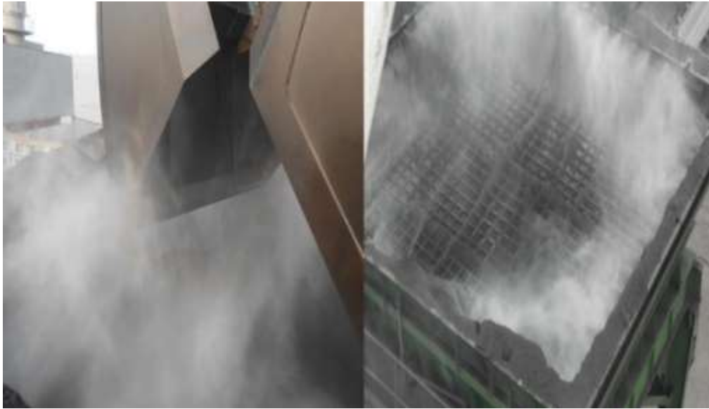
Figure 1: Water fogging system at work at the unloading hopper
