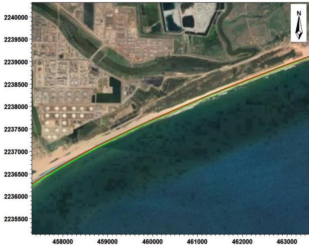
Figure 2-10 Shoreline change at Zone-2. Baseline conditions after 1-year (blue colour), Layout condition after 1-year (red colour) and Layout condition after 5-years (green colour)
