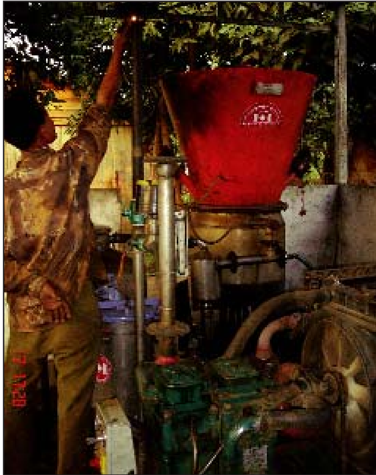
A Biomass Gassifier in Anlong Tamey, Battambang. Photo courtesy of SME Renewable Energy Ltd.
