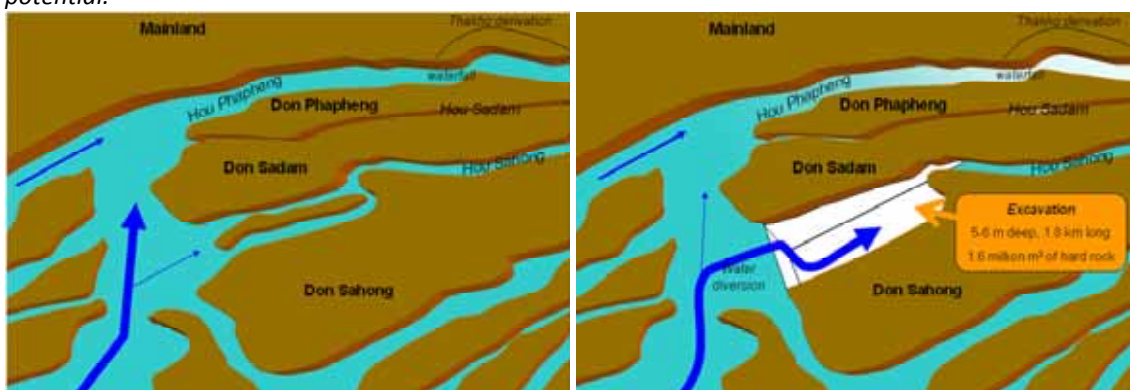
Figure 38: Proposed Don Sahong channel excavation: 1.6 million tonnes would be excavated from the Hou Sahong channel to encourage a greater proportion of the dry season flow and enhance electricity generation potential.
