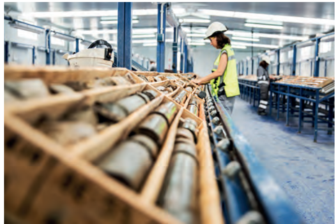
Inspection of core samples, MATSA mine, Spain.
